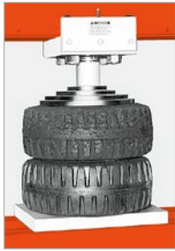
Pressing rim into new tire on Power Team Press.
