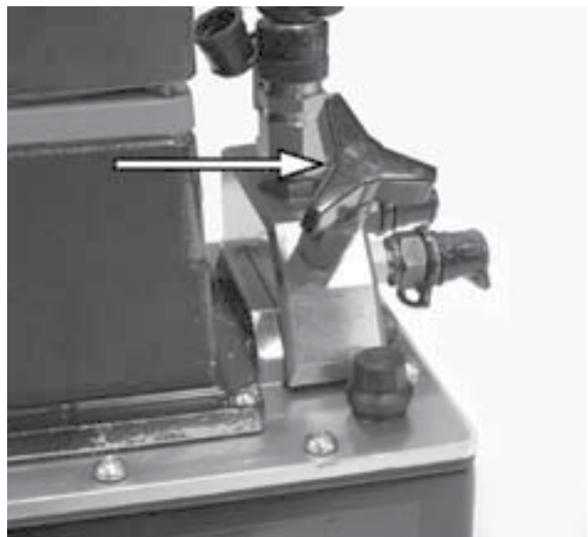
Figure 25. Pressure Regulating Valve
