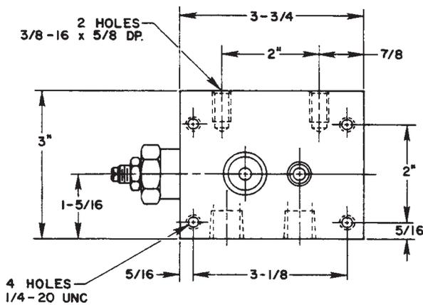
For remote mounting of 3-way and 4-way manual valves. The built-in pressure regulating valve is adjustable to any pressure between 1,000 PSI and 10,000 PSI. Mounting holes are provided for surface or side mounting.
