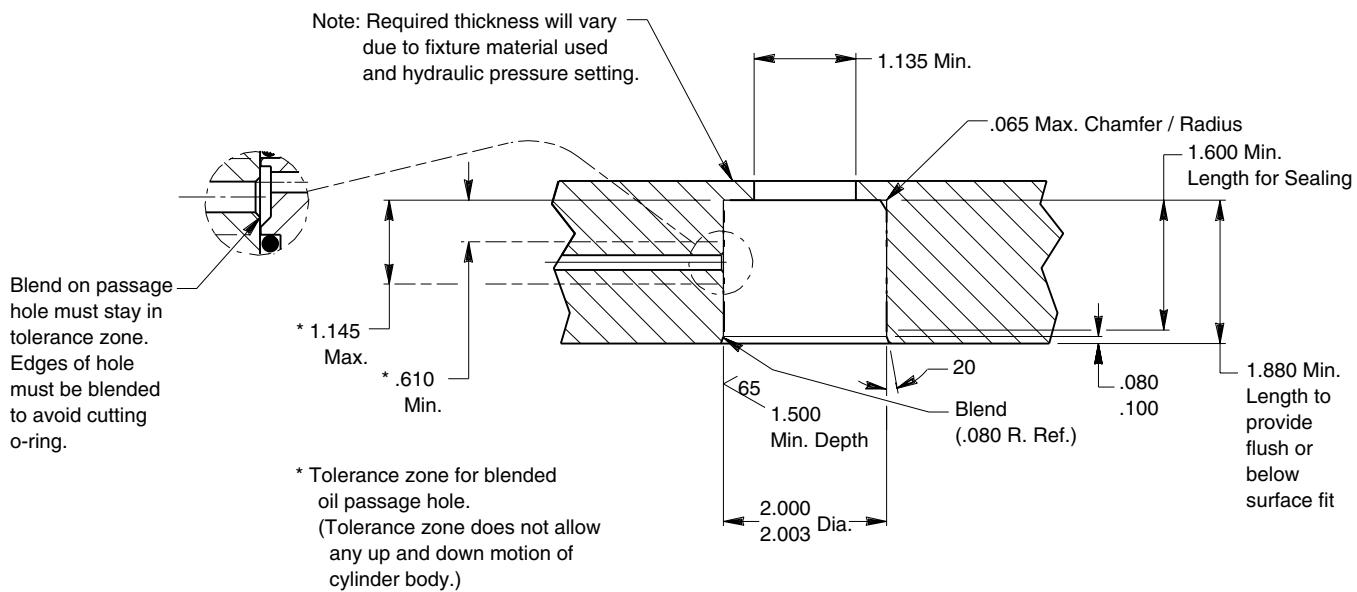
**Cylinder in mounting cavity:**
