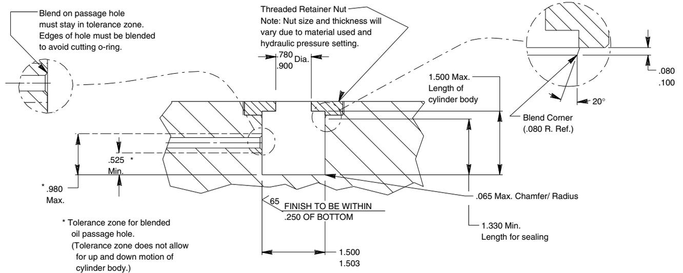
Cylinder in mounting cavity:
