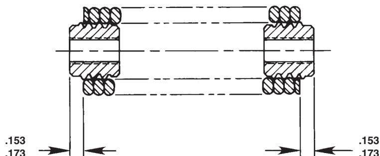
Spring must not extend beyond threads of spring retainer on either end. Stretch, clean and lubricate before assembly.
