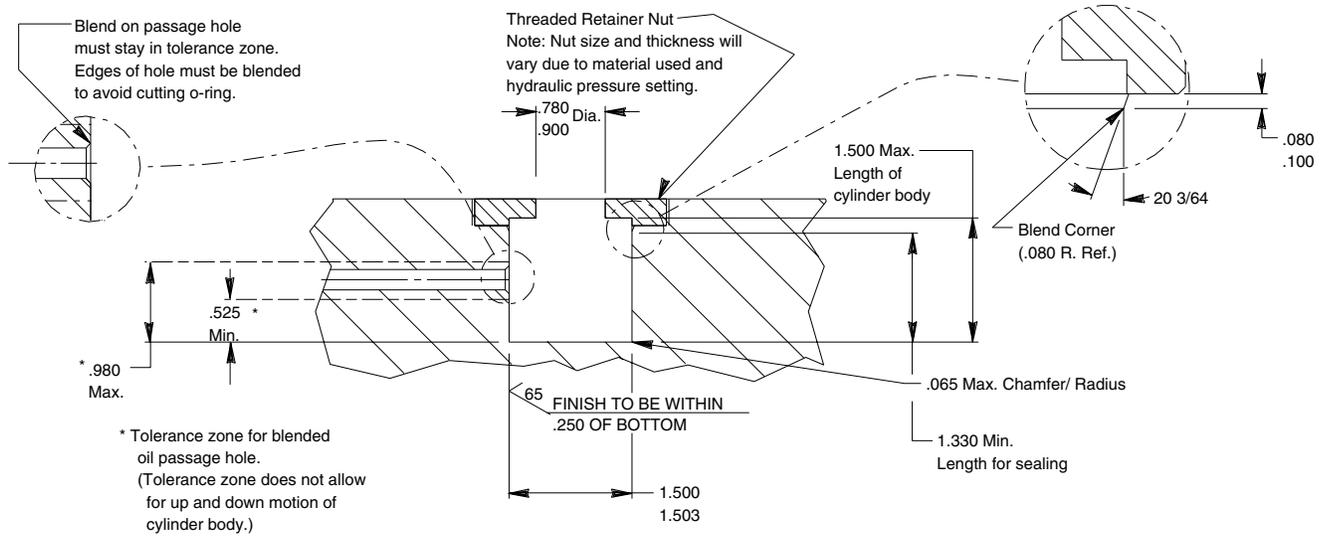
**Cylinder in mounting cavity:**
