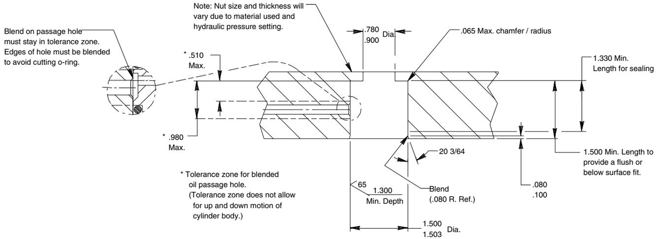
Cylinder in mounting cavity:
