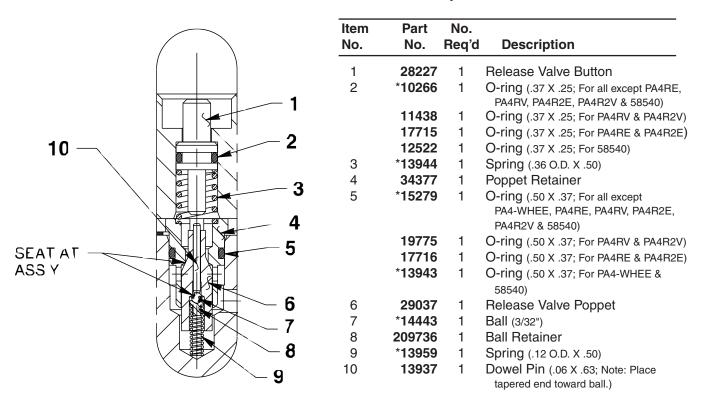
Part numbers marked with an asterisk (\*) are contained in a repair kit. See back sheet 9 of 10 for individual repair kit information.
