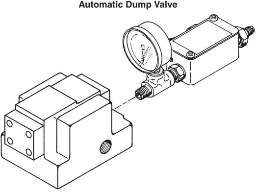
When the pressure switch setting is reached, the switch shuts off the motor. All pressure is automatically dumped. Turn the adjusting screw clockwise to increase pressure. Turn the adjusting screw counterclockwise to decrease pressure. Refer to the section titled "Adjusting the Pressure Switch for further information.
