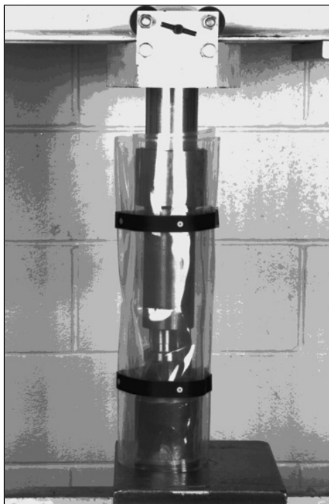
Blanket covers the housing, the bearing being installed, and the installing tool.
