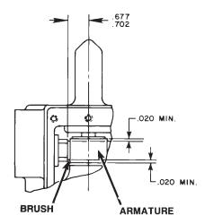
When replacing brushes or the armature, the dimensions shown must be as specified.
